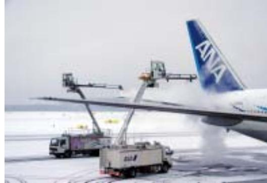
Low-noise type de/anti-icing vehicle (New Chitose Airport)
