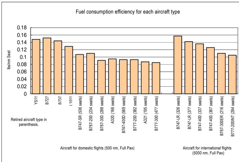
Fig. 2-5 Fuel consumption efficiency of each aircraft type
