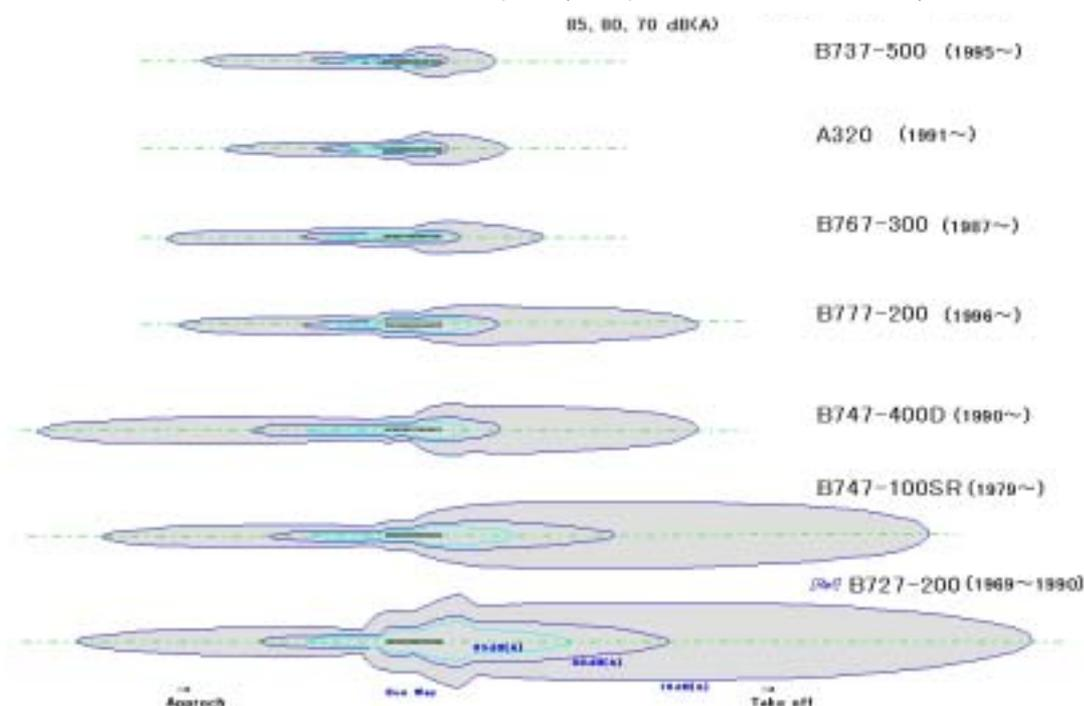
Fig. 4-3 Comparison of noise contour by aircraft type
