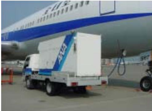
Low-noise type AC Electrical Power Supply Car
