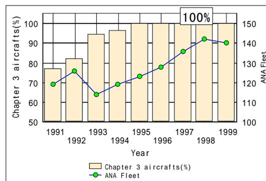
Fig.2-1 ANA fleet that conform to Chapter 3 standards
